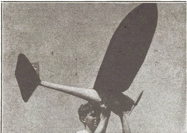
Kenneth Fisher, New York modeler, with his combination power plane-glider. Timer action retracts and extends landing gear wheel. Note polyhedral tail. Fuselage is planked and nose cowling removable.
