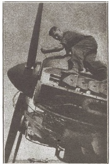
Last-minute adjustments. Before a test flight, Dzus-type fasteners are twisted and metal cowls are locked in place. Note large exhaust ports on Daimler-Benz.
