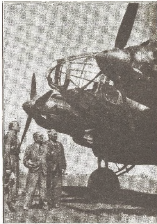
Professor Heinkel inspects the new ship before its maiden flight. With him are Chief Engineer and test pilot. Note generous panelling of the gunner-bombardier's station in the ship's nose.
