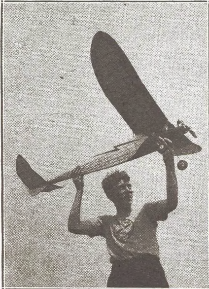
Another unidentified shot of a modeler who undoubtedly will recognize himself. His Ohlsson-powered polyhedral-flyer is also a good soarer. Note the absence of main rudder.
