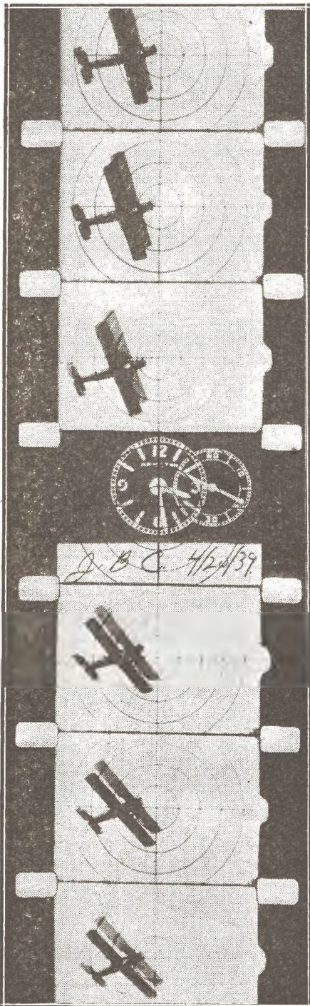
Below: Enlargement of strip of 16mm. film from a gun camera. Image of stopwatch is photographed at end of each burst of fire.
